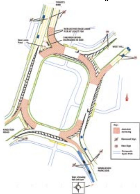
Proposed layout for A3 roundabout in Wandsworth Reproduced by permission of Wandsworth Borough Council
